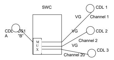
The customer requests that the voiceband circuit serving CDL 3 be moved from channel 20 in the DS1 serving CDL A to Channel 3 in the same DS1. No NRCs apply for this request.
