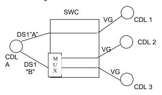
The customer requests that the voiceband (VG) circuit serving CDL 1 be moved from the DS1 "A" circuit to the DS1 "B" circuit. No NRCs apply for this request.
