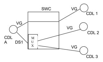
The customer requests that the voiceband circuit (VG) between CDL A and CDL 1 be "rolled over" to the DS1 servingCDL A. No NRCs apply for this request.
