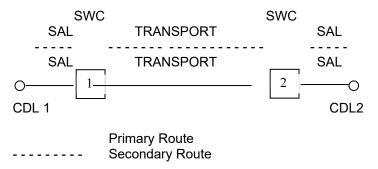
Two diverse circuits between serving wire centers. The SAL and Transport facilities must be separate, although the SWC's may be the same.
